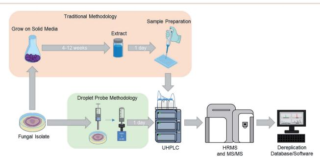
Fig. 1 For traditional screening of fungal cultures for drug discovery purposes, the initial analysis may occur after growing a fungal culture for approximately 6–12 weeks (top). Using the droplet probe, the chemistry of cultures is evaluated much sooner and directly from the Petri dish (bottom), opening the door for examining a suite of different growth conditions both readily and rapidly. Adapted from Sica et al.<sup>39</sup>
