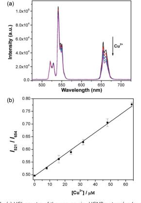
Fig. 5 (a) UCL spectra of the apo-azurin–UCNP system (under excitation from a 980 nm laser) in the presence of varying concentrations of  ${\rm Cu}^{2+}$  ions; (b) the ratio ( ${\rm I}_{521}/{\rm I}_{654}$ ) of UCL intensities of the sensor system at 521 and 654 nm as a function of  ${\rm Cu}^{2+}$  concentration.
