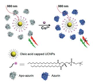
Fig. 1 Schematic illustration of the ratiometric upconversion luminescence sensing of Cu<sup>2+</sup> based on an azurin–UCNP biosensor.
