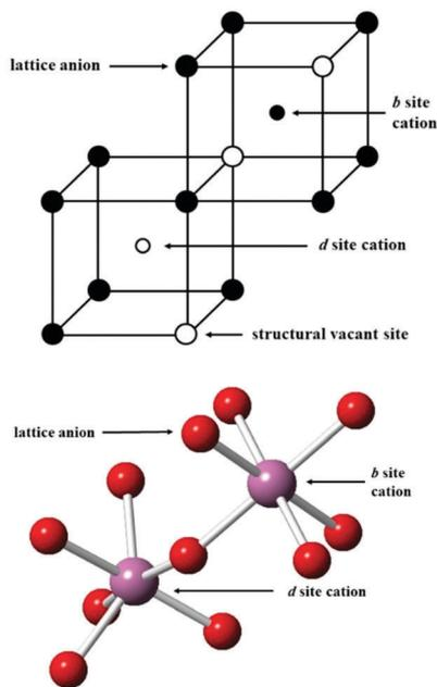
Fig. 1 Lattice sites in  $\text{In}_2\text{O}_3$ . In the bottom figure, the coordination of the cations is shown, with indium ions represented by larger purple spheres and oxygen ions by smaller red spheres.
