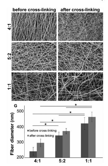
Fig. 1 (A-F) SEM images of electrospun GE: PLA at different ratios before (A, C and E) and after cross-linking (B, D and F). (G) Fiber diameter comparison among the hybrid GE:PLA electrospun scaffolds. \* $p \le 0.05$ .
