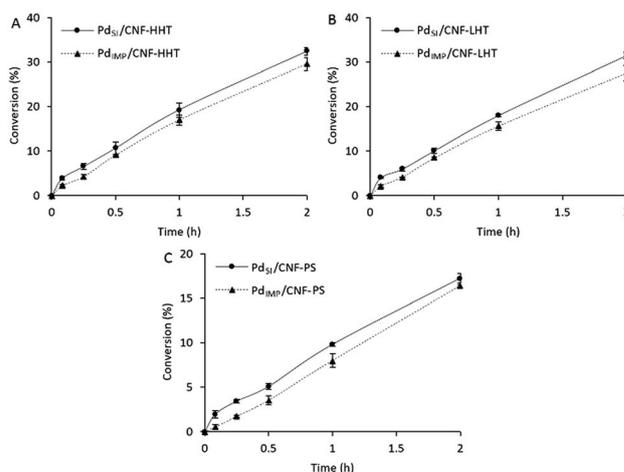
**Fig. 9** Formic acid dehydrogenation reaction on (A) Pd/CNF-HHT, (B) Pd/CNF-LHT, and (C) Pd/CNF-PS. Comparison of preparation methods.
