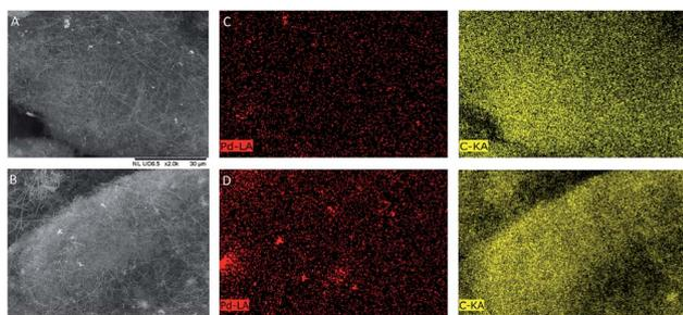
**Fig. 8** (A) SEM image of fresh Pd<sub>IMP</sub>/CNF-HHT, (B) SEM image of used Pd<sub>IMP</sub>/CNF-HHT, (C) mapping images of fresh Pd<sub>IMP</sub>/CNF-HHT, and (D) mapping images of used Pd<sub>IMP</sub>/CNF-HHT.
