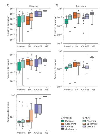
Fig. 3 Average smallest relative deviations between objectives sampled by different optimization algorithms after 100 objective function evaluations averaged over 25 different optimization runs. Panel (A) reports results on the Fonseca benchmark set, and panel (B) displays results for the Viennet variant benchmark set.
