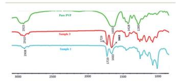
Fig. 5 Infrared spectrum of PVP and PVP/p(HEMA-co-BA) material.
