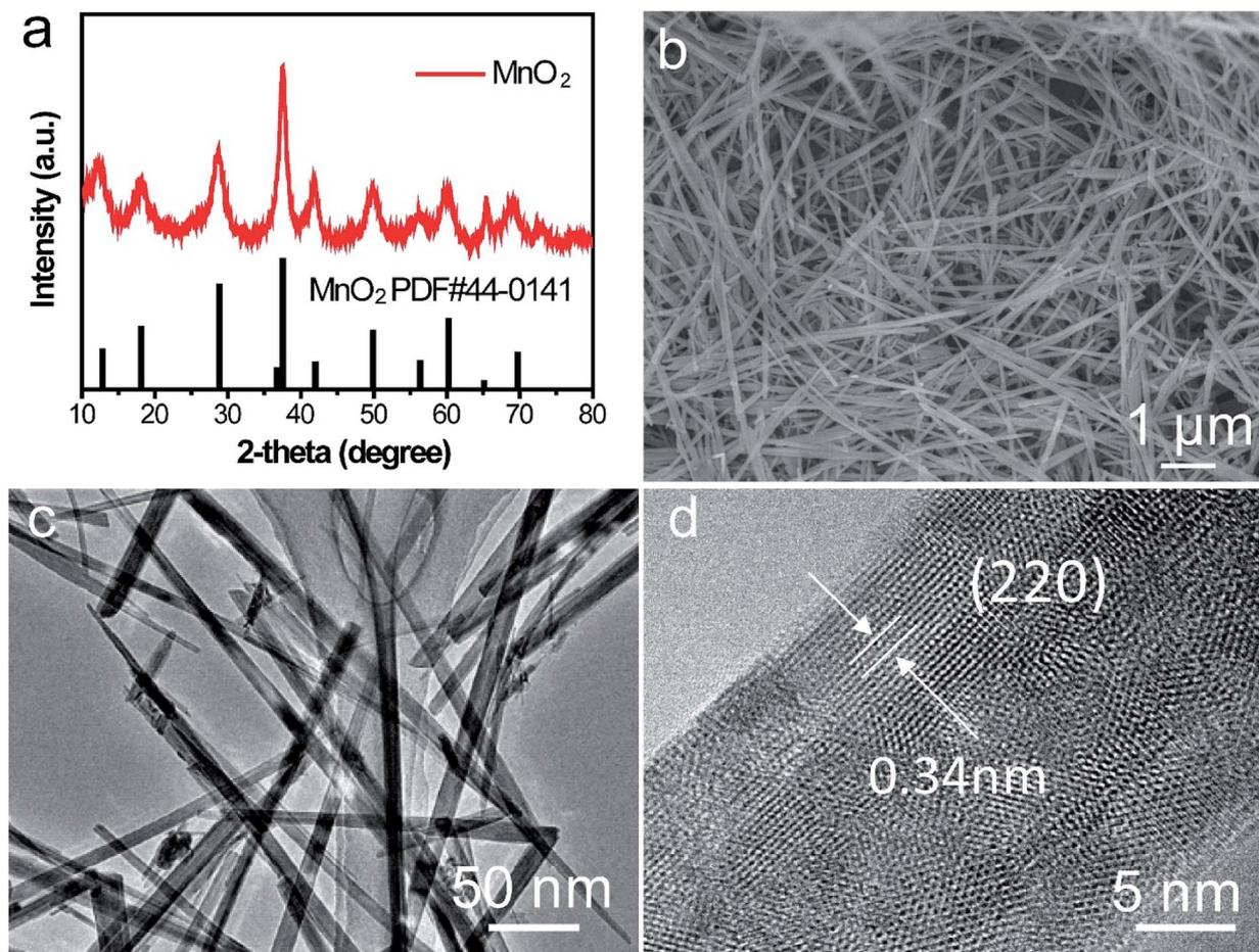
Fig. 5 Characterizations of  $\alpha$ -MnO<sub>2</sub> nanowire cathode. (a) XRD patterns of the as-prepared  $\alpha$ -MnO<sub>2</sub>, (b) SEM image, (c) TEM image and (d) magnified TEM image.
