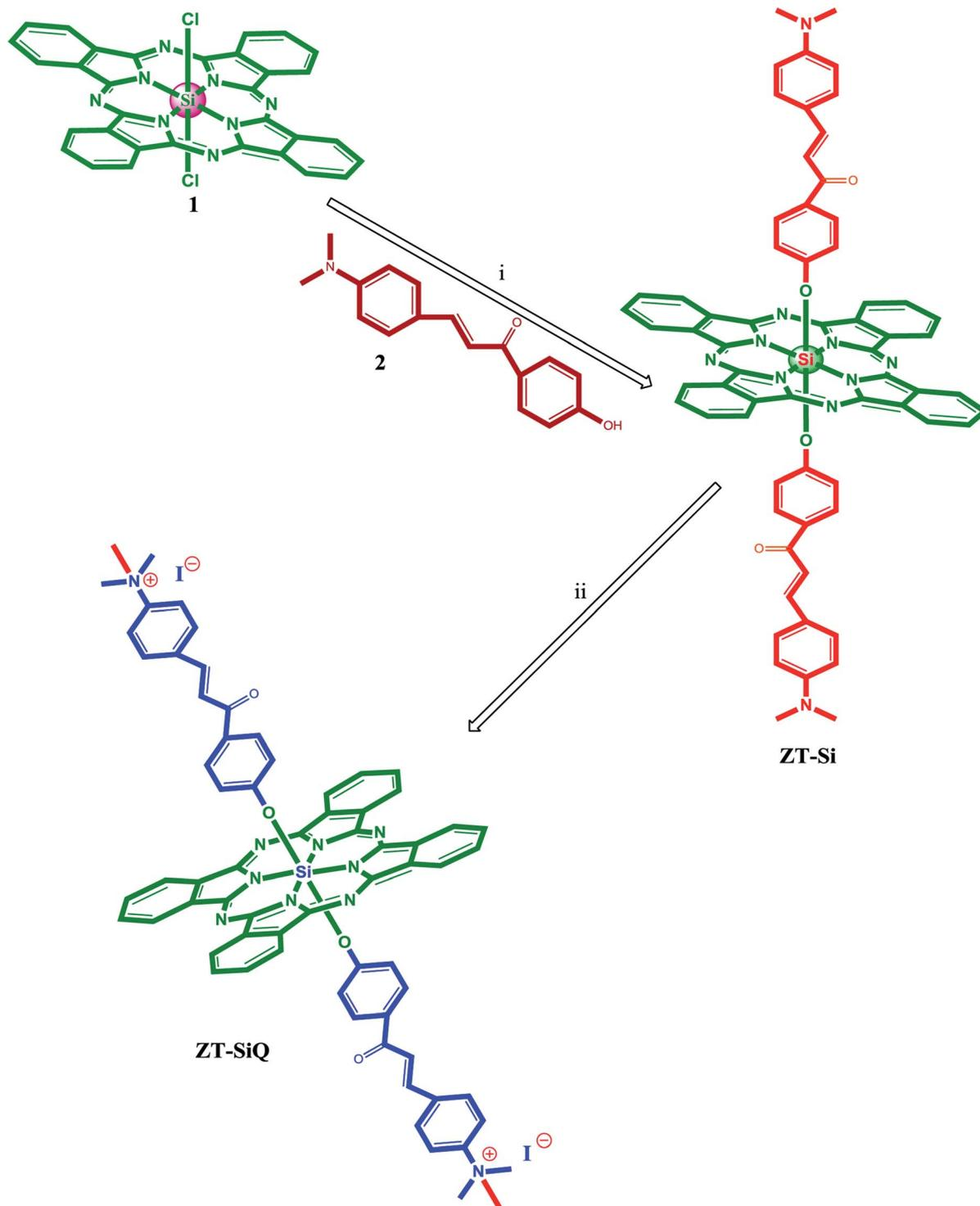
Fig. 2 The synthesis of the silicon(IV) phthalocyanine ZT-Si and its quaternized derivative ZT-SiQ. (i) Toluene, NaH, reflux. (ii) CHCl<sub>3</sub>, CH<sub>3</sub>-I, room temperature.
