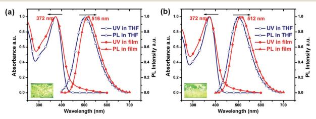
Fig. 1 Normalized absorption and PL spectra of (a) PTPA1-TPE and (b) PTPA2-TPE in dilute THF solution ( $10^{-5}$  M) and as spin-coated films (measured at room temperature). The insets in (a) and (b) show fluorescent images of PTPA1-TPE and PTPA2-TPE powders under UV irradiation, respectively.
