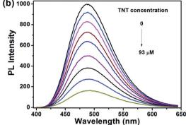
Fig. 3 PL spectra of (a) PTPA1-TPE and (b) PTPA2-TPE in 9:1 (v/v) water/THF solution containing different amounts of TNT. Polymer concentration:  $10^{-5}$  M.
