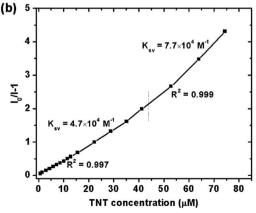
Fig. 5 Stern-Volmer plots of the relative PL intensities of (a) PTPA1-TPE and (b) PTPA2-TPE ( $I_0/I-1$ ) vs. TNT concentration (I: PL intensity,  $I_0$ : PL intensity at zero TNT concentration).
