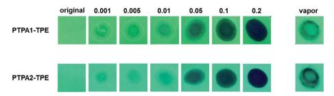
Fig. 7 Paper test strips impregnated with PTPA1-TPE or PTPA2-TPE before and after dropping TNT solutions in THF onto them (concentration: 0.001, 0.005, 0.01, 0.05, 0.1 and 0.2 mg mL<sup>-1</sup>, respectively), and after storage above TNT vapor for 5 min.
