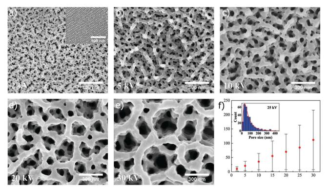
Fig. 3 Tuning the porosity of the resulting pore network during ion beam exposure of superstructures composed of nanospheres, by controlling the ion beam voltage at a constant dose of 0.5 nC  $\mu$ m $^{-2}$ . (a-e) Show SEM micrographs of the resulting pore network after ion beam exposure at 2, 5, 10, 20 and 30 kV, respectively. (f) The measured pore sizes were fitted to a lognormal distribution, and mean values were found to increase in a linear manner with increasing ion beam voltage
