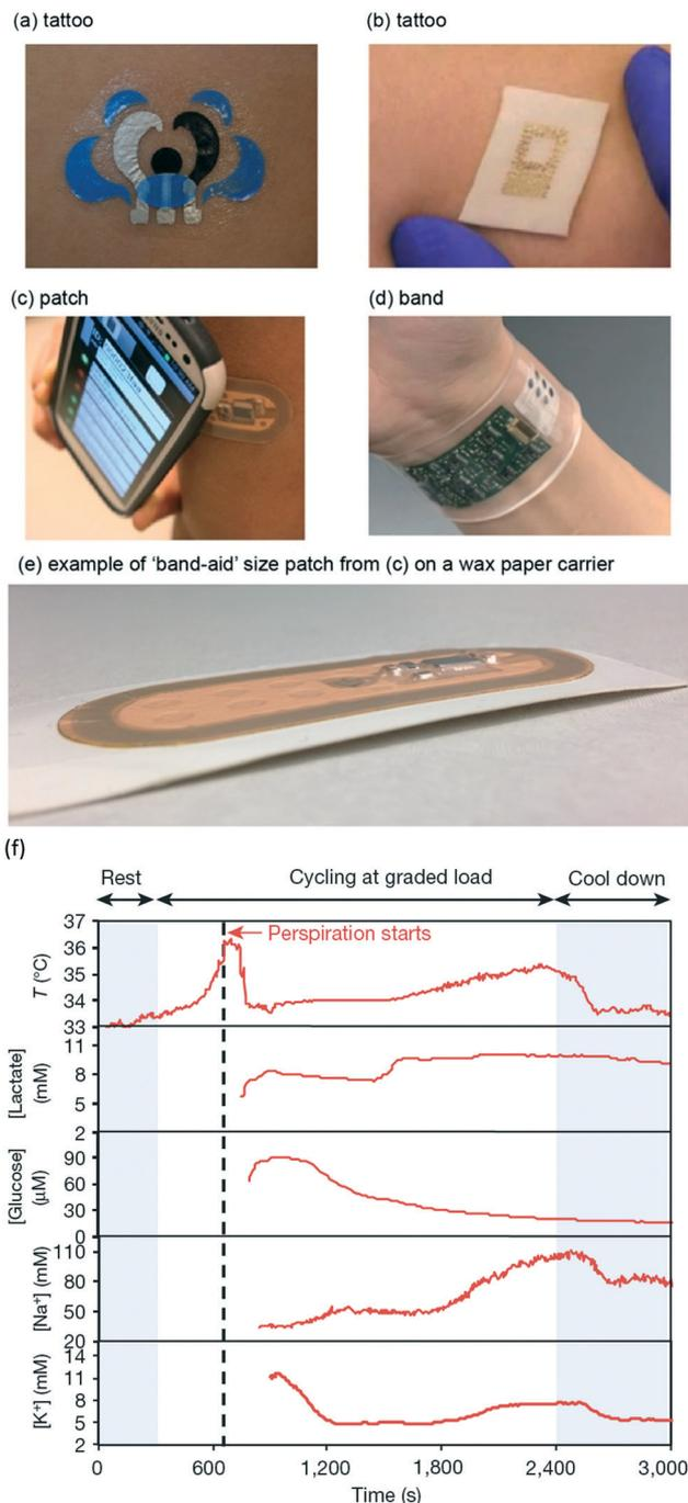
**Fig. 17** Bringing electrochemical sensors directly onto skin to detect sweat (adapted).<sup>158</sup> In all the examples provided in the figure, technology is mechanically compliant to skin, which is a first step to reduce the sweat volume between skin and sensors. The data shown in (f) is for a human subject wearing the technology shown in (d).<sup>178</sup>
