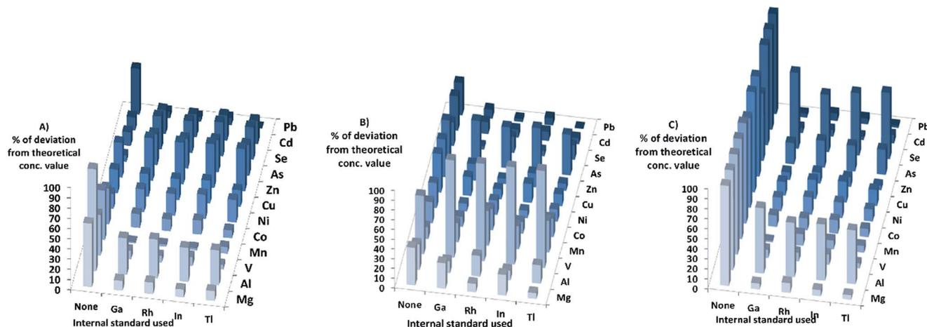
Fig. 4 Highest absolute deviation from theoretic concentration values for all matrix compositions in DRC-mode, when using 1% HNO<sub>3</sub>-matrix for calibration. Scale restricted to a maximum of 100% deviation. (A) HNO<sub>3</sub>, (B) PBS, (C) Triton.
