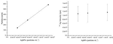
Fig. 1 External calibration with AgNPs. (Left) Measured number of AgNP events *versus* AgNP concentrations (equation: number of AgNP events  $= 0.0040 \times [\text{AgNPs mL}^{-1}] - 2.90$ ;  $R^2 = 0.999$ ). (Right) Measured <sup>107</sup>Ag in counts per second (cps) *versus* AgNP concentrations.
