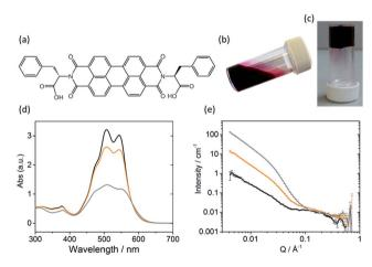
Fig. 1 (a) Molecular structure of PBI-F; (b) high pH solution (10 mg mL<sup>-1</sup> PBI-F, 2 eq. NaOH, 20 v/v% methanol); (c) low pH gel (10 mg  $mL^{-1}$  PBI-F, 2 eq. NaOH, 8 mg  $mL^{-1}$  GdL, 24 hours); (d) UV-Vis absorption spectra and (e) SANS data at pH 11 (black), 6 (orange), and 2 (grey), pH was lowered in (d) by HCl addition and in (e) by DCl addition.
