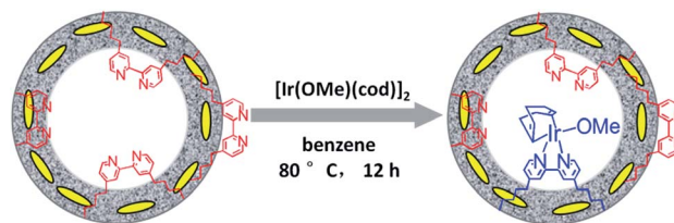
Scheme 3 Synthetic route for the molecular heterogeneous solid catalyst \text{Ir}(\text{cod})\text{-BPY}_{0.3}\text{-NT} .
