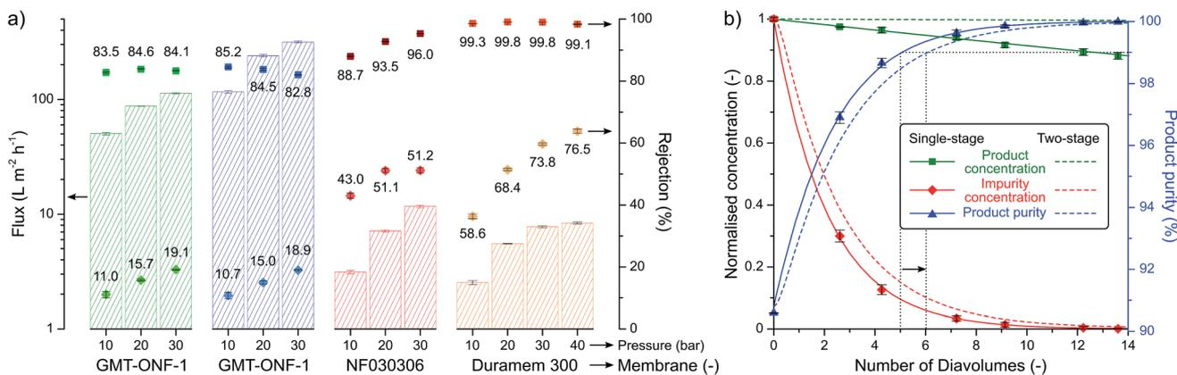
**Fig. 6** Separation performance of the solvent-resistant nanofiltration membranes for 2-imidazoline product purification: ■ and ◆ indicates rejections for **1**, and the corresponding benzaldehyde substrate impurity, respectively (a). Purification performance for single-stage and two-stage diafiltration processes. Solid and dashed lines represent the simulated performance based on rejections, while symbols signify experimental points to validate the model used for simulation (b).
