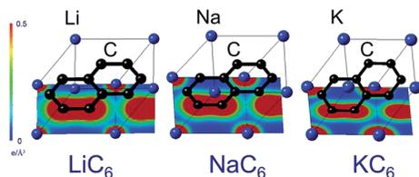
Fig. 3 Electron densities for compositions  $\text{LiC}_6$ ,  $\text{NaC}_6$  and  $\text{KC}_6$  plotted to the same scale. For  $\text{KC}_6$  and  $\text{NaC}_6$ , the electron density between C and AM atoms is negligibly small. For  $\text{LiC}_6$ , in contrast, the electron density between C and Li is greater, indicating some covalency in the bonding between C and Li. This covalent contribution stabilizes Li-GIC layers, despite the small size of the Li atom.
