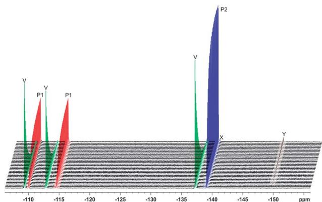
Fig. 3  $^{19}\text{F}$  NMR spectra during a 17 h alkaline stress test, showing the consumption of voriconazole (V), the formation of major degradation products 1 (P1) and 2 (P2), and minor degradation products X and Y. Spectra are shown at half hour intervals.
