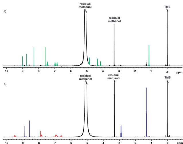
Fig. 2  $^1\text{H}$  NMR spectra of alkaline stress testing; (a) time 0, and (b) after 17 h. Signals shown in green are from voriconazole, in red from degradation product 1, and in blue from degradation product 2, both here and in subsequent figures.
