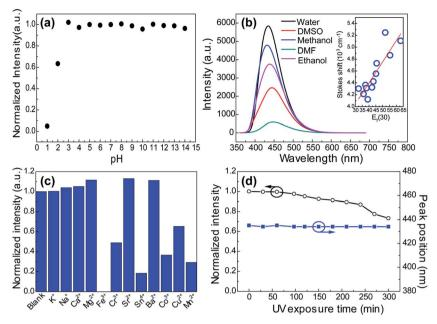
Fig. 7 The effect of pH (a), solvent (b), metal ions (c), and UV exposure (d) on the fluorescence intensities of CACDs. Inset in (b): the Stokes shift were compared to published values of  $E_T(30)$ , a measure of microscopic solvent polarity.
