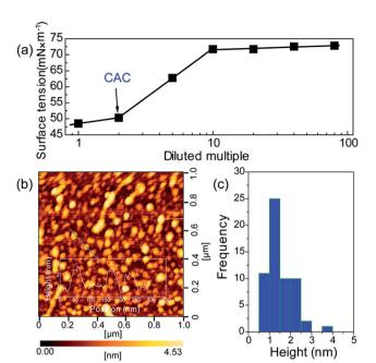
Fig. 4 (a) Surface tension of the mixed solution of DETA and CA at the concentration of 10 mg  $\rm mL^{-1}$  with diluted multiple at 25 °C micelle formation. (b) AFM topography image of CA–DETA mixed systems and sectional height profile along the line shows inset. (c) Height distribution estimated from (b).
