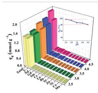
Fig. 5 Effect of pH on the extraction of U(vi) in a multi-ion system ( $C_0 \approx 1.0$  mmol L $^{-1}$  for all cations, t=120 min, v=25 mL, T=298 K, and  $\omega=10$  mg), the inset shows the uranium-selectivity ( $S_U$ ) of HSOF towards uranium at different pH values.
