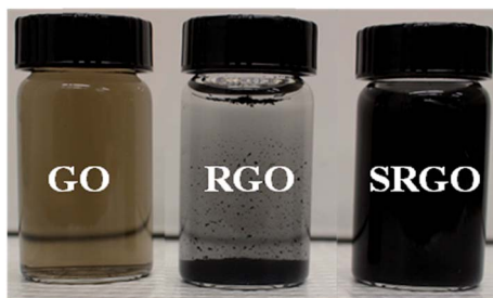
Fig. 1 Optical images of GO, RGO and SRGO dispersed in water at the concentration of 0.5 mg \text{mL}^{-1} .
