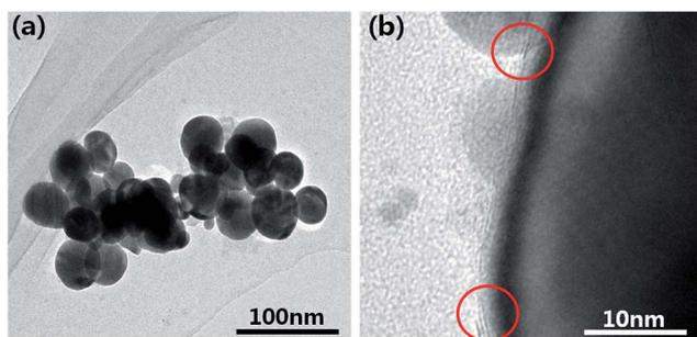
Fig. 4 (a) TEM image of the MoS<sub>2</sub>@AgNPs structure. (b) TEM image of the MoS<sub>2</sub>@AgNPs structure in high magnification.
