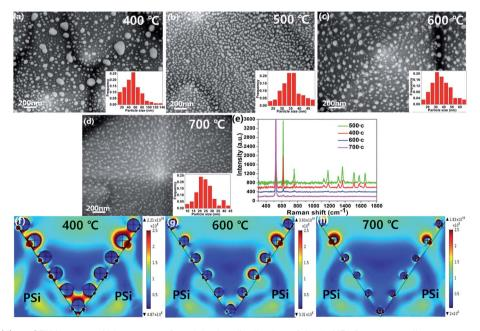
Fig. 7 (a), (b), (c) and (d) are SEM image and histograms of particle size distribution of the AgNPs for an annealing temperature at 400 °C, 500 °C, 600 °C and 700 °C, respectively. (e) Raman spectra of R6G molecules that the concentration is  $10^{-6}$  M on the AgNPs@PSi substrate with different annealing temperature from 400 °C to 700 °C. (f), (g) and (h) are the electric field distribution of the AgNPs@PSi substrate at 400 °C, 600 °C and 700 °C, respectively.
