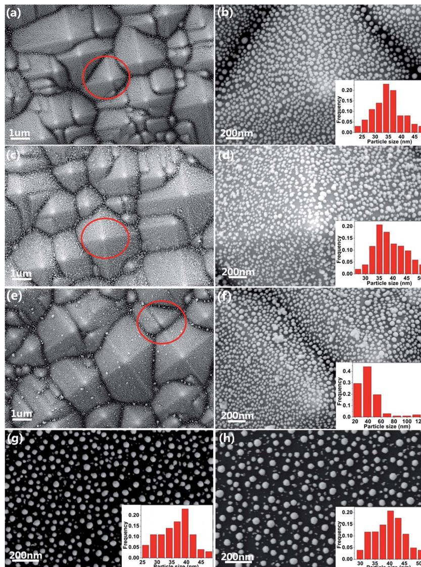
Fig. 2 (a) and (b) are SEM images of the AgNPs@PSi substrate in different magnification. (c) and (d) are SEM image of the MoS<sub>2</sub>@AgNPs@PSi substrate in different magnification. (e) and (f) are SEM images of the AgA@PSi substrate in different magnification. (g) SEM image of the AgNPs@flat-Si substrate. (h) SEM image of the MoS<sub>2</sub>@AgNPs@flat-Si substrate.
