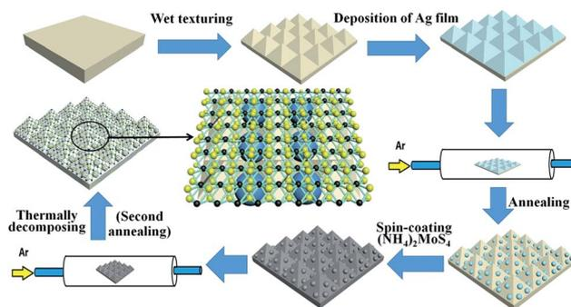
Fig. 1 The preparation processes of the MoS<sub>2</sub>@AgNPs@PSi substrate.
