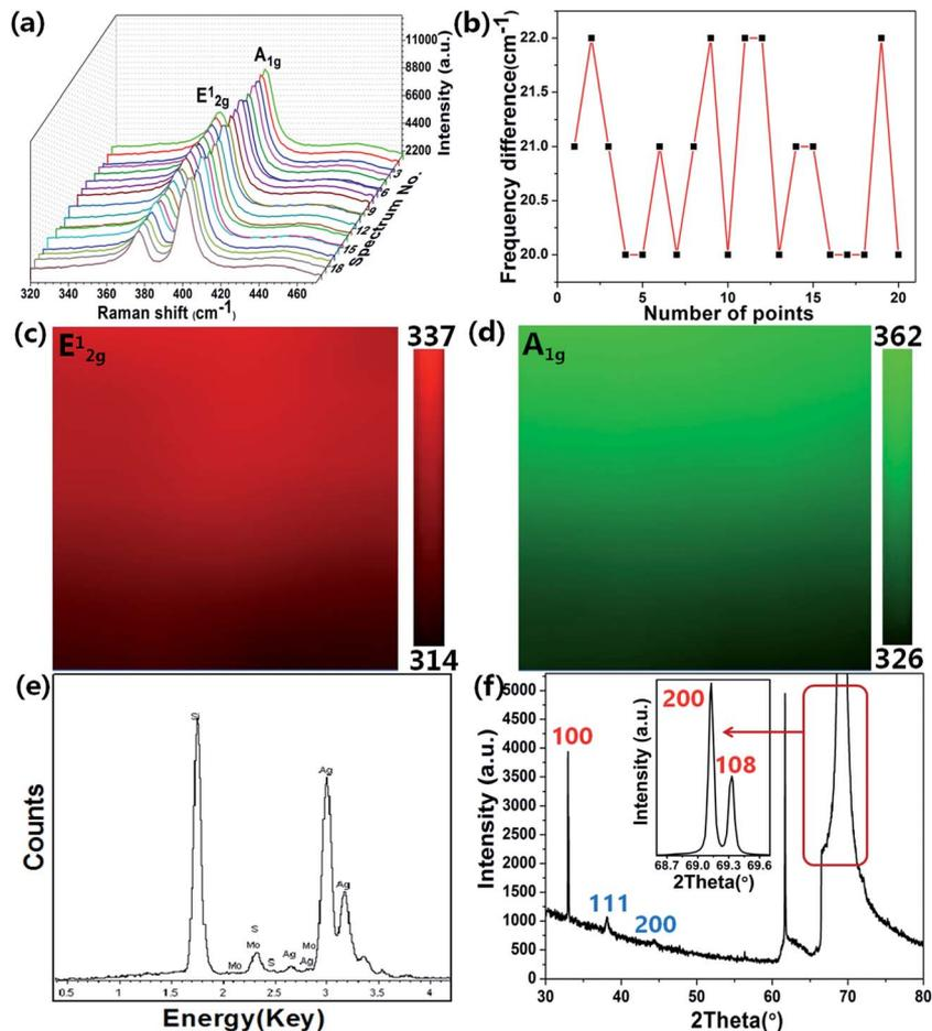
Fig. 3 (a) Raman spectra of the MoS<sub>2</sub> layers from the MoS<sub>2</sub>@AgNPs@PSi substrate. (b) The calculated peak frequency difference ( $\Delta$ ) between E<sub>2g</sub> and A<sub>1g</sub> Raman modes according to the Raman spectra in (a). (c) and (d) are Raman mapping of E<sub>2g</sub> and A<sub>1g</sub> peaks of MoS<sub>2</sub>, respectively. (e) EDS spectra of the MoS<sub>2</sub>@AgNPs@PSi substrate. (f) XRD pattern of the MoS<sub>2</sub>@AgNPs@PSi substrate.
