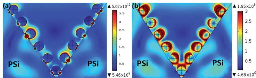
Fig. 6 (a) The electric field distribution of the AgNPs@PSi substrate. (b) The electric field distribution of the MoS<sub>2</sub>@AgNPs@PSi substrate.
