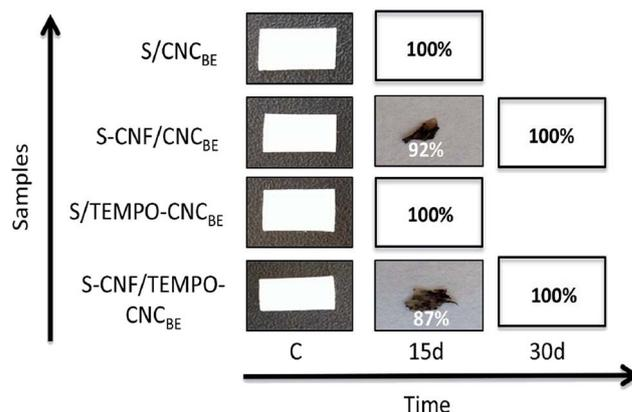
Fig. 8 Photographs from different stages of degradation in waste water and soil. Complete degradation was recorded for unmodified membranes within 15 days.
