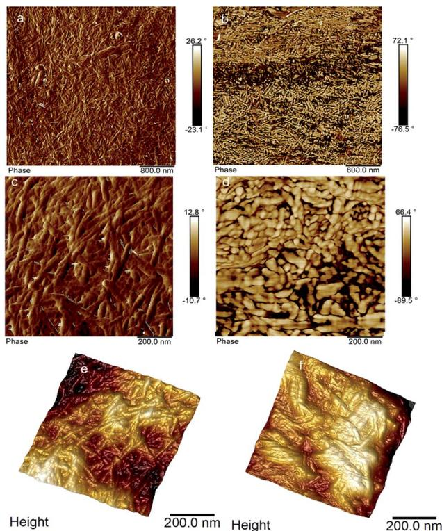
Fig. 4 AFM images of the top layer of the membranes before and after *in situ* modifications. (a and c) Shows the phase images at different magnifications and (e) shows the 3D height images of CNC<sub>BE</sub> layer. (b, d and f) Shows the corresponding phase images at different magnifications and the 3D height images of CNC<sub>BE</sub> layer after *in situ* TEMPO modification.
