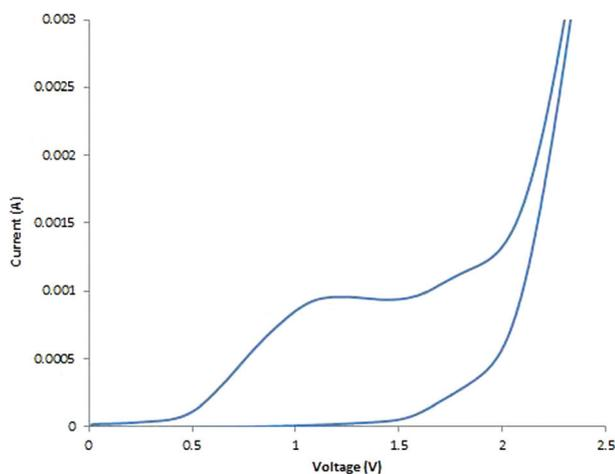
**Fig. 2** Cyclic voltammetry measurement on substrate **1a** (5 mM) at a scan rate of  $10 \text{ mV s}^{-1}$  in 9 : 1 acetonitrile : methanol and TBAP (0.5 M) using an RVC working electrode, RVC counter electrode and a Ag/AgCl reference electrode.
