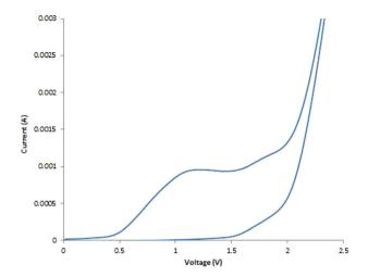
Fig. 2 Cyclic voltammetry measurement on substrate 1a (5 mM) at a scan rate of 10 mV s<sup>-1</sup> in 9:1 acetonitrile: methanol and TBAP (0.5 M) using an RVC working electrode, RVC counter electrode and a Ag/AgCl reference electrode.
