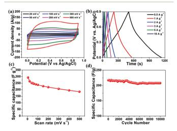
Fig. 8 (a) CV curves at different scan rates. (b) Charge–discharge curves at current densities ranging from 0.5 to 10 A  $\rm g^{-1}$ . (c) Specific capacitance curves at the different scan rates from 20 to 500 mV s<sup>-1</sup>. (d) Variation of the specific capacitance within 10 000 cycles at the scan rate of 100 mV s<sup>-1</sup>.
