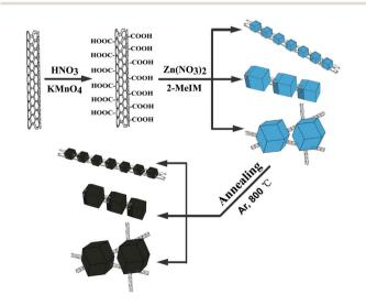
Fig. 1 Synthetic scheme for the fabrication of MWCNT/NPC-S/M/L.
