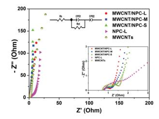
**Fig. 9** Nyquist plots of MWCNT/NPC-S/M/L, NPC-L, and MWCNTs, the insets show an equivalent circuit consisting of two constant phase elements CPE1 and CPE2 (upper), and an expanded view for the high-frequency range (bottom).
