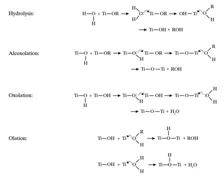
Fig. 5 Hydrolysis and condensation reactions leading to titanium dioxide formation. Curved arrows indicate nucleophilic attack and the transition state.
