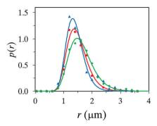
Fig. 7 Size distribution of microcapsules produced with propellant pressures of 2.8 ( $\bigcirc$ ), 2.0 ( $\triangle$ ), and 1.4 ( $\bigcirc$ ) bar.
