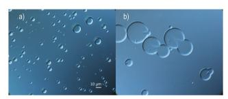
Fig. 4 (a) Optical micrograph of microcapsules loaded with oleyl alcohol using 1 wt% PVA in water phase. (b) Optical micrograph of typical instability of larger microcapsule where broken and fractured microcapsules are shown with their inner core released out to the surrounding. Scale bar is valid for both micrographs
