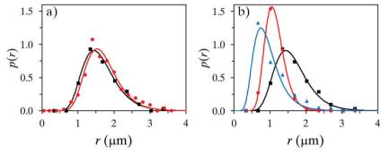
Fig. 3 (a) Size histograms and fitted lognormal distributions of microcapsules loaded with pure oleyl alcohol using 1 wt% PVA in the water phase ( compared to using pure water (a). (b) Size histograms and fitted lognormal distributions of the microcapsules (1 wt% PVA) directly after formulation (1). one week after formulation ( ), and one month after formulation ( ).
