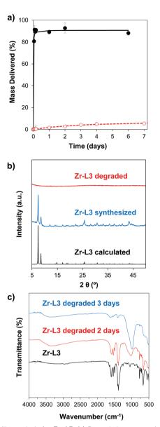
Fig. 3 Stability analysis for Zr-L3. (a) Degradation pattern in PBS (black closed dots) and H<sub>2</sub>O (red open dots). (b) PXRD patterns of calculated Zr-L3 (black), synthesized (blue) and samples incubated for 2 days in PBS (red). (c) FTIR analysis after PBS exposure for 0 days (black), 2 days (red) and 3 days (blue).
