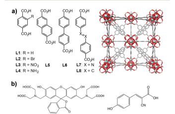
Fig. 1 (a) Chemical structure of the organic linkers used to synthesize the different Zr-based MOFs (left) and packing structure of Zr-L6 (right); (b) chemical structure of guest molecules, calcein (left) and  $\alpha$ -CHC (right).
