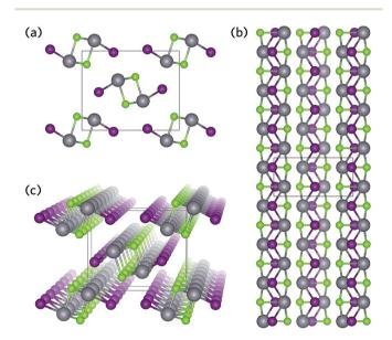
Fig. 1 Crystal structure of BiSel as viewed along (a) the [100] direction, (b) the [001] direction, and (c) a three-dimensional view, highlighting the 1D chains. Bi, Se, and I atoms are denoted by grey, green, and purple spheres, respectively.
