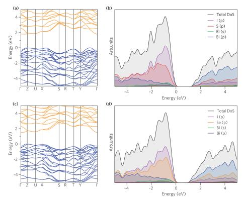
Fig. 3 (a and c) Band structures along the high symmetry directions, and (b and d) ion decomposed partial and total density of states, for BiSI and BiSel, respectively. In all cases the valence band maximum is set to zero eV. The valence bands and conduction bands of (a and c) are denoted by blue and orange respectively
