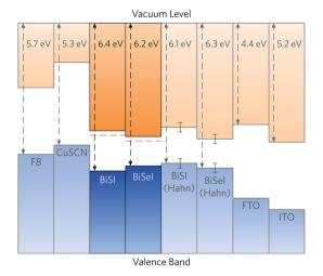
Fig. 5 Calculated band alignment of BiSI and BiSeI with a range of hole transporting materials and transparent conducting oxides, taken from experiment. <sup>85–90</sup> The CBM alignments from the HSE06 calculated VBM energy levels and extrapolated using the experimental band gaps are shown in dashed red lines. Alignments calculated from experiment by Hahn *et al.* are also included, with the experimental error indicated. <sup>42</sup>
