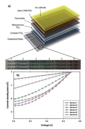
Fig. 5 (a) Device structure, (b) photocurrent density-voltage (J-V)curve of the fabricated solar cells with transparent graphene electrodes. PSC devices with 0.075 cm<sup>2</sup> active area were illuminated under AM 1.5G simulated sunlight (100 mW cm $^{-2}$ ).
