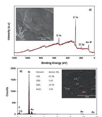
Fig. 3 (a) XPS survey spectra (inset: SEM image of AuNPs-RGO) and (b) EDX analysis (red box in the inset is the selected area for analysis) of RGO-SDBS film after  $HNO_3$  and  $HAuCl_4$  treatments.
