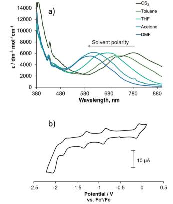
Fig. 1 (a) UV/vis absorption spectra of complex 3 recorded in solvents of different polarity and (b) the cyclic voltammogram of 3 in DMF with  $[^{n}Bu_{4}N][BF_{4}]$  (0.2 M) as supporting electrolyte at a scan rate of 0.1 V s<sup>-1</sup>.
