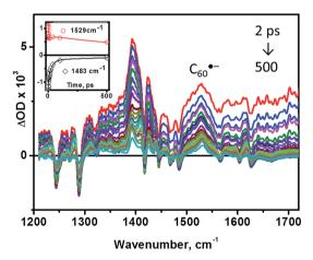
Fig. 4 TRIR spectra of **3** in  $CD_2Cl_2$  solution at 298 K upon laser excitation at 400 nm,  $\sim$ 50 fs pulse, at different time delays. Inset: kinetics at selected frequencies. Symbols are experimental points, and the lines are multiexponential fits to the data using the parameters obtained by a global fit, which yielded lifetimes values of 2.5 ( $\pm$ 0.3) ps, 31 ( $\pm$ 0.4) ps, and 890 ( $\pm$ 17) ps.
