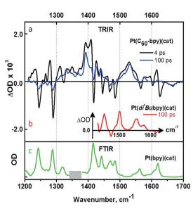
Fig. 5 (a). TRIR spectra of 3 in  $CD_2Cl_2$  at two selected time delays; (b) TRIR spectrum of a model compound 10 (no band at 1530 cm<sup>-1</sup> observed) obtained under identical conditions to (a); (c) FTIR spectrum of compound 10 in  $CH_2Cl_2$ .
