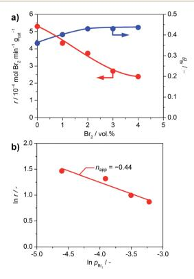
Fig. 7 (a) Rate of bromine formation (red) and bromine surface coverage (blue) *versus* the volumetric feed of bromine over  $TiO_2$  at 593 K and  $O_2$ : HBr = 2. (b) Rate of bromine formation *versus* partial pressure of bromine.
