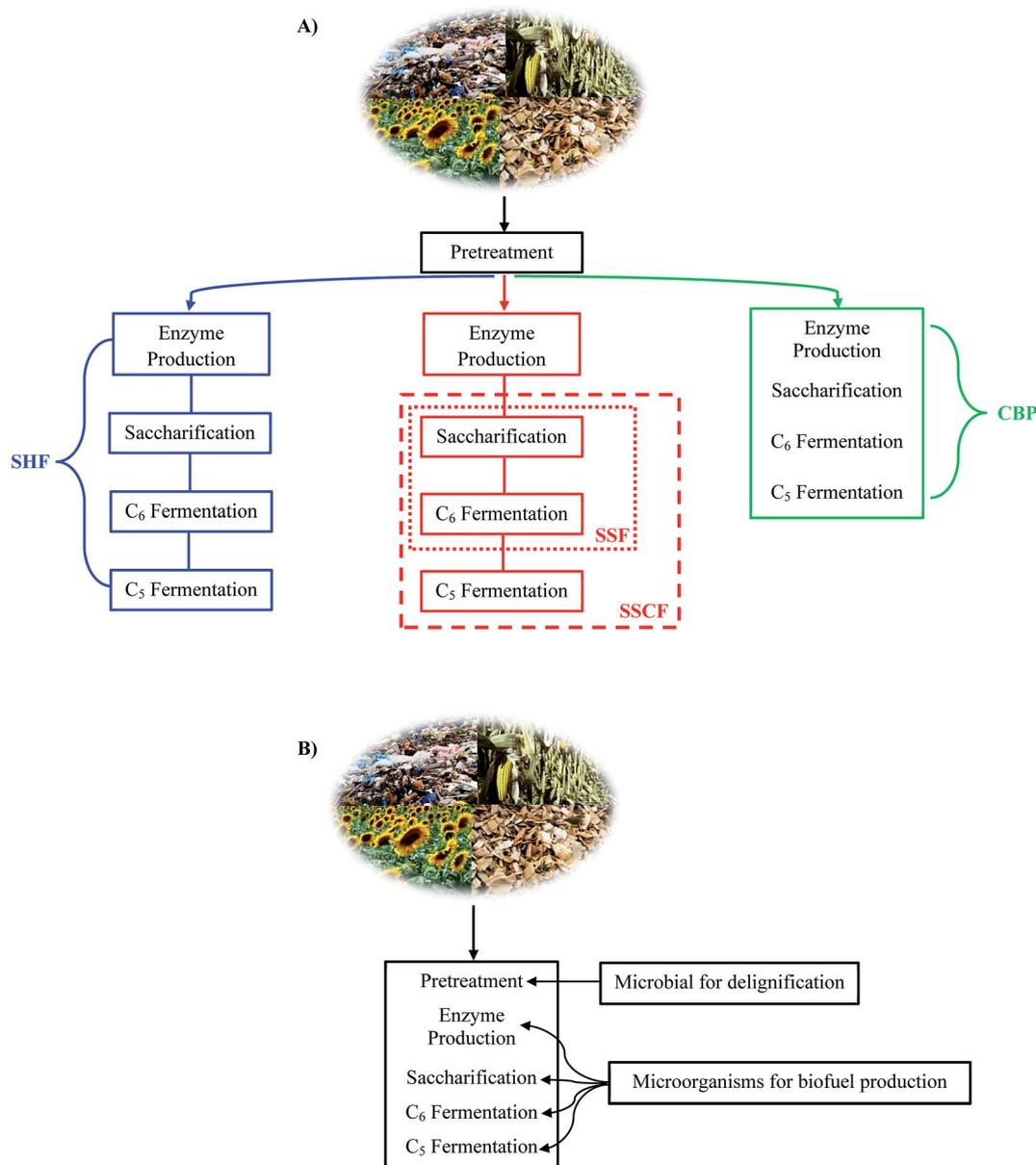
Fig. 4 (A) Schematic process for SHF, SSF/SSCF and CBP (B) schematic process for IBP.
