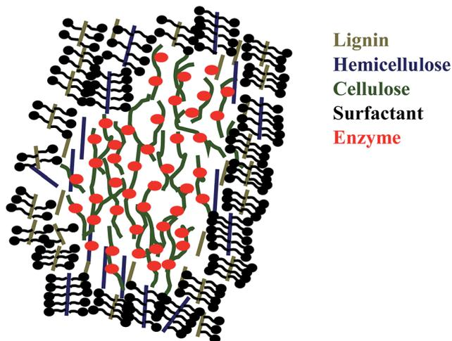
Fig. 3 Scheme of mechanism of surfactant in saccharification.
