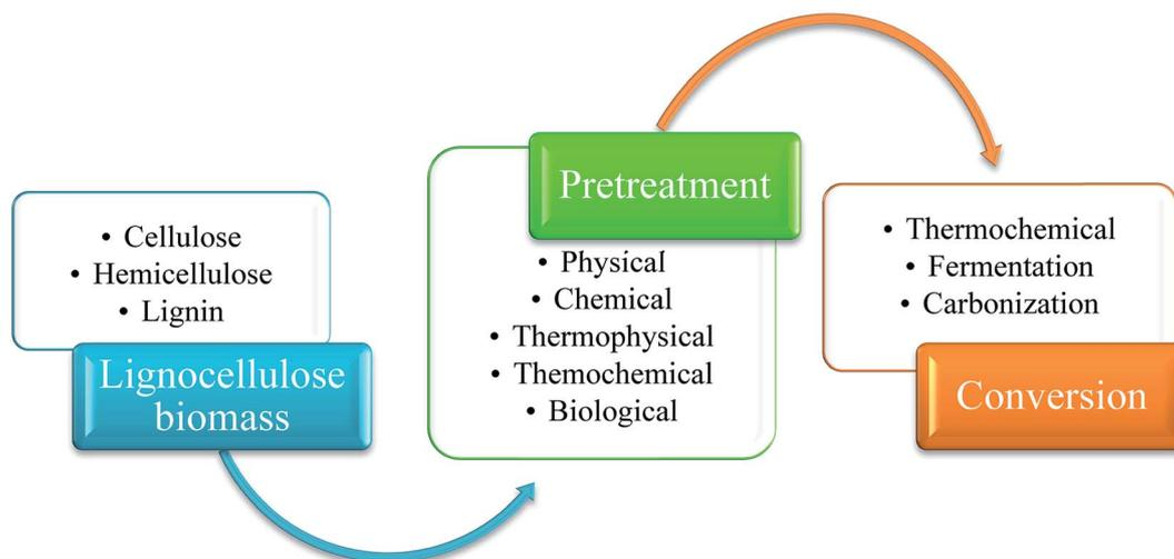
**Fig. 1** Schematic diagram showing utilization of lignocellulose biomass.
