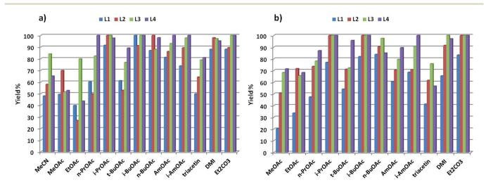
Fig. 1 Catalytic results for the synthesis of aryl ether 1: (a) base =  $Cs_2CO_3$ ; (b) base =  $K_3PO_4$  (GC yields using trimethoxybenzene as internal standard).
