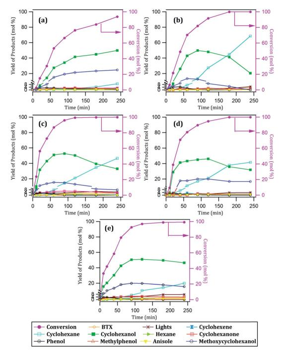
Fig. 4 Conversion of guaiacol and yield of products with time over: (a) 10Ni/CNT, (b) 12Ni/CNT, (c) 15Ni/CNT, (d) 17Ni/CNT and (e) 20Ni/CNT catalysts.
