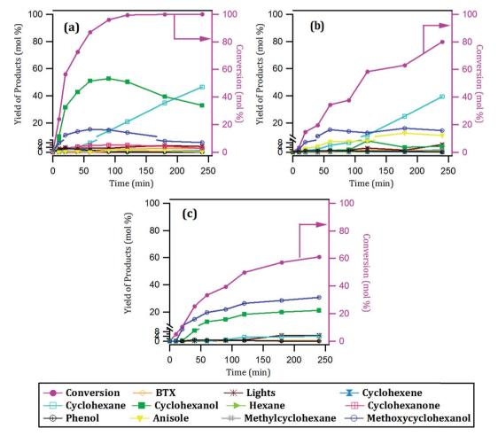
Conversion of quaiacol and yield of products with time over: (a) 15Ni/CNT, (b) 15Ni/CNTox and (c) 15Ni/AC catalysts
