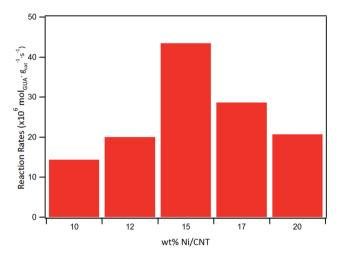
Fig. 7 Initial reaction rate as a function of Ni loading
