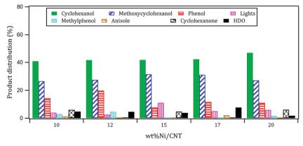
Fig. 6 Products distribution at 20% conversion of quaicol over xNi/CNT catalysts.
