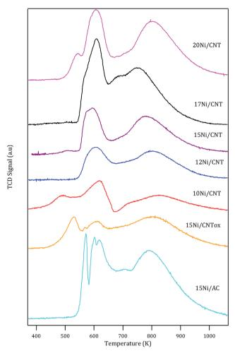
Fig. 1 H<sub>2</sub>-TPR profiles of the supported Ni catalyst
