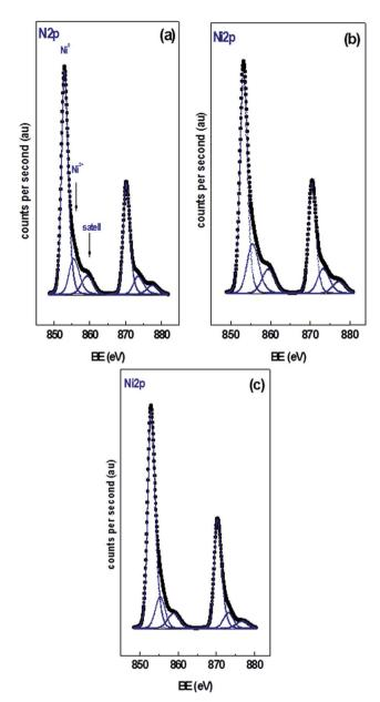
Fig. 2 XPS spectra of the Ni 2p region of (a) 15Ni/CNTox, (b) 15Ni/CNT and (c) 15Ni/AC catalysts.
