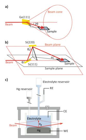
Fig. 2 Liquid interface scattering geometry with (a) a single deflecting crystal and (b) a double crystal Bragg deflector. (c) Electrochemical cell for X-ray scattering studies of liquid metal-electrolyte interfaces. The X-ray beam enters and leaves the cell through glass windows and passes through the bulk of the electrolyte solution before and after reflection at the Hg surface. The entire cell is kept in an inert gas atmosphere to keep the electrolyte clean and free of oxygen.
