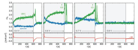
Fig. 6 Kinetic studies of PbFBr growth and dissolution on Hg in 0.01 M NaF + 0.01 M NaBr + 0.25 mM PbBr<sub>2</sub> by *operando* X-ray scattering. Shown is the time dependent behaviour of the specular XRR signal at  $q_z = 0.9 \text{ Å}^{-1}$ , (blue), of the PbFBr (001) Bragg peak (green) and of the simultaneously measured electrochemical current density (red) at four different potentials (after ref. 36).
