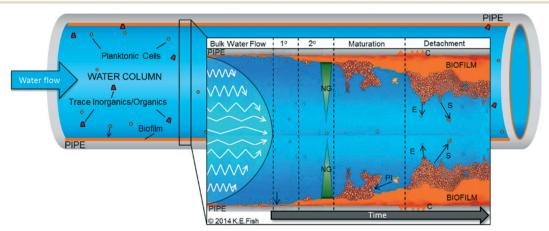
Fig. 1 Biofilm development within DWDS incorporating water flow within the pipe. As the distance from the wall increases the flow becomes more laminar, 1° - primary adhesion, 2° - secondary adhesion, NG - nutrient gradient, concentrates within the biofilm, PI - protozoan interactions, C - corrosion of the pipe surface, E - erosion, S - sloughing.
