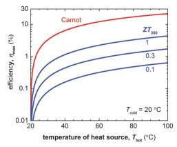
Fig. 15 The Carnot efficiency (red) and maximum efficiency  $\eta_{\rm max}$  of a thermoelectric leg (blue) with increasing heat source temperature  $T_{\rm hot}$  (the heat sink is kept at  $T_{\rm cold}$  = 20 °C). Eqn (8) was used to calculate  $\eta_{\rm max}$  for materials with a figure of merit at 300 K of  $ZT_{300}$  = 0.1, 0.5 and 1.
