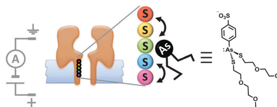
Fig. 18 Stochastic walking of a small molecule within a transmembrane nanopore. 40
