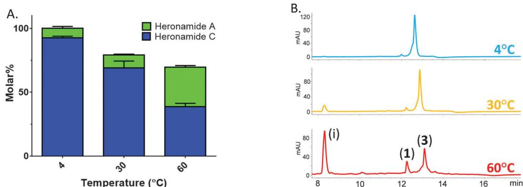
Fig. 3 Temperature sensitive conversion of heronamide C (**3**) to heronamide A (**1**) after seven days of incubation: (A) the proportion of **1** and **3** as a molar percentage of the starting material; and (B) a section of the HPLC trace showing **1**, **3** and the main decomposition product (i) (for full chromatograms see Fig. S6, ESI†).
