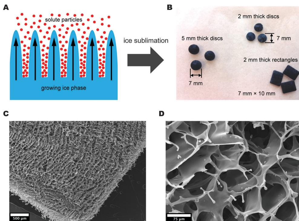
**Fig. 1** (A) Schematic showing the ice templating process. (B) Photograph of PEDOT:PSS scaffolds made from molds of various shapes. Rectangular scaffolds were used in this work. (C) Low magnification SEM image of a PEDOT:PSS scaffold prepared in a PTFE mold from 1.25 wt% PEDOT:PSS dispersion with 3 wt% GOPS at a controlled freezing rate. (D) Higher magnification SEM image of a PEDOT:PSS scaffold, showing the macroporous architecture generated by ice-templating.
