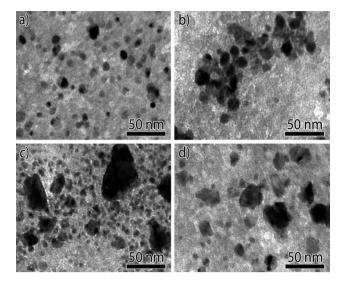
Fig. 8 TEM images of Ni/SiO $_2$  catalysts with different Ni particle sizes after 150 h on-stream (230 °C, H $_2$  : CO =2 : 1, 0.1 MPa). (a)  $\sim\!8$  nm, (b)  $\sim\!9$  nm, (c)  $\sim\!4$  nm, and (d)  $\sim\!3$  nm. Reproduced with permission from ref. 66 Copyright (c) [2014 WILEY-VCH Verlag GmbH & Co. KGaA, Weinheim].
