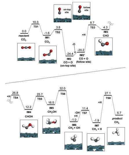
Fig. 12 Potential energy diagram for carbon dioxide methanation on the Ru surface slab structure. Each reactant, product and intermediate structures are also shown in the inset of the figure. Reproduced with permission from ref. 224 Copyright (2014), with permission from Elsevier.
