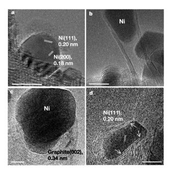
Fig. 6 Electron micrographs of the Ni catalyst and carbon nanofibres. (a) TEM image of a Ni nanocrystal supported on MgAl $_2$ O $_4$ . (b) TEM image showing a multi-walled tubular carbon nanofibre structure. (c) In situ TEM image showing a whisker-type carbon nanofibre. (d) In situ TEM image showing a Ni nanocrystal during carbon nanofibre growth. Scale bars, 5 nm. Reprinted by permission from Macmillan Publishers Ltd: [Nature] (ref. 84), Copyright (2004).
