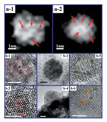
Fig. 5 (a-1 and a-2) High-angle annular dark field (HAADF) STEM images of Ni nanoparticles in Ni/H-Al<sub>2</sub>O<sub>3</sub>. (b-1-b-6) HRTEM images of Ni nanoparticles selected from the Ni/H-Al<sub>2</sub>O<sub>3</sub> sample (the scale bar is 2 nm). Reprinted with permission from ref. 52 Copyright (2013) American Chemical Society.
