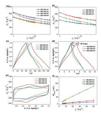
Fig. 6 Electrochemical performance comparisons of carbon materials activated at various conditions based on the three-electrode system: (a and b) C<sub>s</sub> at various current densities; galvanostatic charge/ discharge curves collected at (c) 5 A g<sup>-1</sup> and (d) 50 A g<sup>-1</sup>; (e) CVs at 200 mV  $s^{-1}$ ; (f)  $IR_{drops}$  collected at various current densities.
