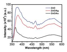
Fig. 2 Room temperature photoluminescence spectra of ZnO, ZnO/Au, and ZnO/Ag nanoparticles. All the powder samples were well dispersed in water using a sonicator for PL measurements using an excitation wavelength ( $\lambda_{\rm ex}$ ) of 325 nm.
