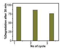
**Fig. 12** Percentage of degradation *vs.* number of cycle plot for ZnO/Au nanoparticles after 30 min exposure under a visible light source. The catalyst particles were centrifuged and washed well before each cycle of use.
