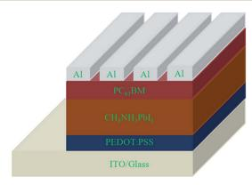
Fig. 1 Structure of CH<sub>3</sub>NH<sub>3</sub>PbI<sub>3</sub>/PC<sub>61</sub>BM solar cells.
