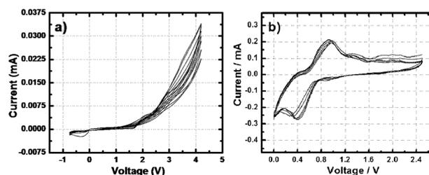
Fig. 2 Typical cyclic voltammograms of Al-ion battery using  $\text{V}_2\text{O}_5$  nano-wire cathode and aluminium anode in (a) 1:1 v/v of Al triflate in PC/THF and (b) 1.1:1 molar ratio of  $\text{AlCl}_3$  in  $([\text{EMIm}]\text{Cl})$  at a sweep rate of  $0.2$   $\text{mV s}^{-1}$ .
