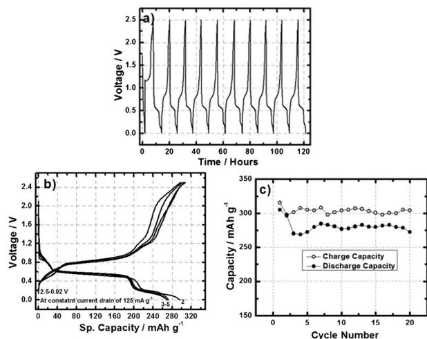
**Fig. 3** (a) Voltage vs. time (b) voltage vs. sp. capacity and (c) cycle life plot of Al-ion battery containing aluminium anode, V<sub>2</sub>O<sub>5</sub> nano-wire cathode in ionic liquid under the potential window 2.5–0.02 V and at a constant current drain of 125 mA g<sup>-1</sup>.
