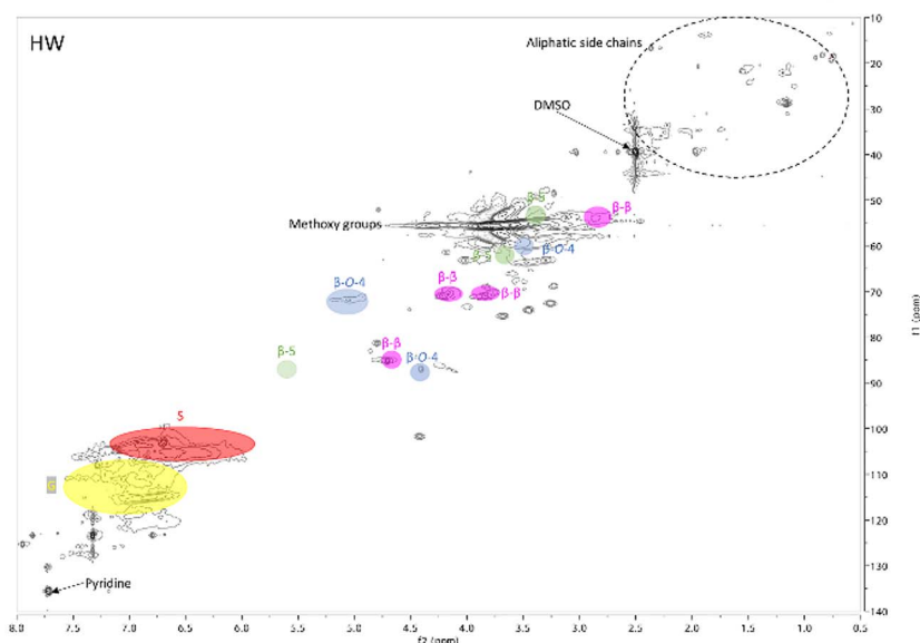
Fig. 1 HSQC spectrum of (a) softwood lignin (SW) and (b) hardwood lignin (HW).
