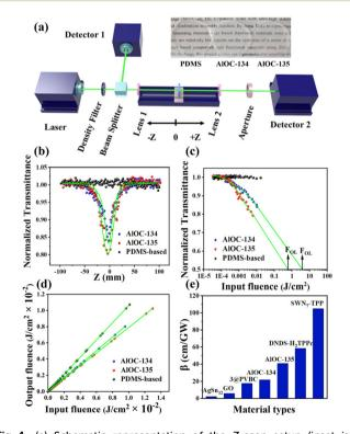
Fig. 4 (a) Schematic representation of the Z-scan setup (inset is a picture of the PDMS substrate and AlOCs@PDMS under natural light); (b) the OA Z-scan curves of input laser pulse energy 80  $\mu J$  of AlOCs@PDMS: (c) the plots of normalized transmittance versus input fluence; (d) curves of output fluence versus input fluence; and (e) the plots of comparisons of the nonlinear absorption coefficients.
