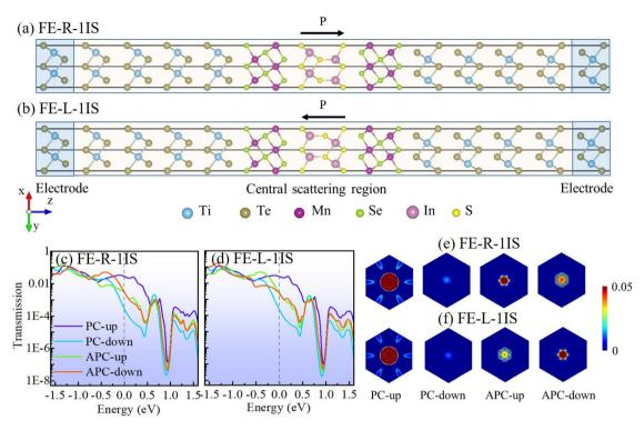
Fig. 2 The structure schematic diagrams of the MFTJ with (a) FE-R-1IS and (b) FE-L-1IS states. The spin-dependent zero-bias transmission coefficient curves of the MFTJ with (c) FE-R-1IS and (d) FE-L-1IS states. The spin-dependent  $k_{\parallel}$ -resolved transmission spectra of the MFTJ with (e) FE-R-1IS and (f) FE-L-1IS states.
