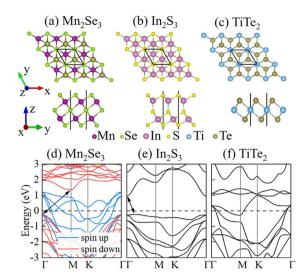
Fig. 1 The top and side views of the crystal structures of (a)  $Mn_2Se_3$ , (b)  $In_2S_3$  and (c)  $TiTe_2$  monolayers. The band structures of (d)  $Mn_2Se_3$ , (e)  $In_2S_3$  and (f)  $TiTe_2$  monolayers.
