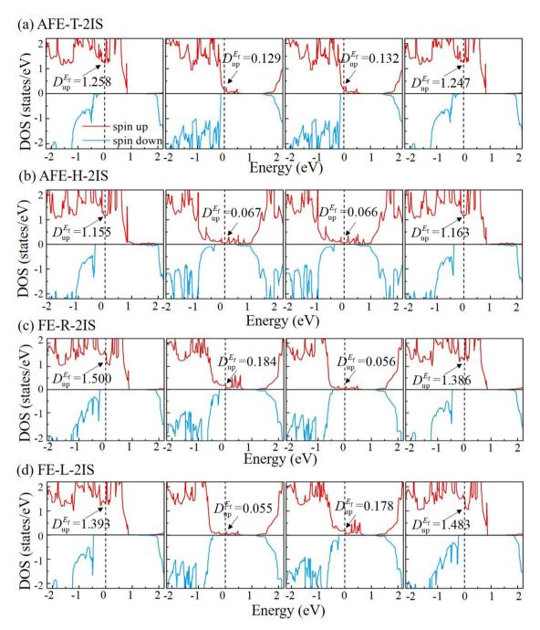
Fig. 5 The spin-dependent DOS of the Mn<sub>2</sub>Se<sub>3</sub>/bilayer-In<sub>2</sub>S<sub>3</sub>/Mn<sub>2</sub>Se<sub>3</sub> part in the MFTJ with (a) AFE-T-2IS, (b) AFE-H-2IS, (c) FE-R-2IS and (d) FE-L-2IS states.  $D_{\rm up}^{\rm Ef}$  represents the spin-up DOS value at the Fermi level.
