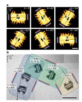
Fig. 4 Magnetic manipulation of a soft polymeric microrobot. (a) Controlled rotational motion of a fluorescent microrobot in a glycerol/ distilled water mixture (50/50 vol%). Scale bar, 100 µm. In the stitched image sequence (b), the navigation of a microrobot along a 90-degree curved pathway using external magnetic field guidance and acoustic propulsion (f = 23.3 kHz,  $V_{PP} = 22.5 \text{ V}$ ) is shown. Scale bar, 500  $\mu$ m.
